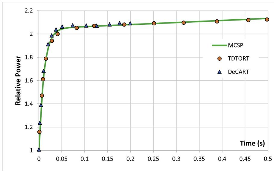
Fig. 8. The relative power vs. time for the step transient in the TWIGL transient problem.
