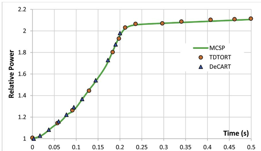
Fig. 9. The relative power vs. time for the ramp transient in the TWIGL transient problem.
