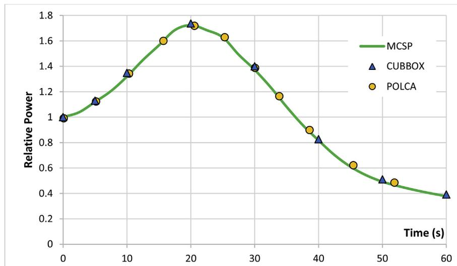
**Fig. 12.** The relative power vs. time for the LMW transient without feedback.
