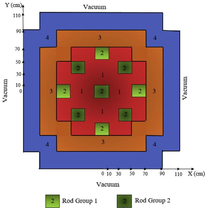
Fig. 10. Schematic of the LMW core layout on the X-Y page.
