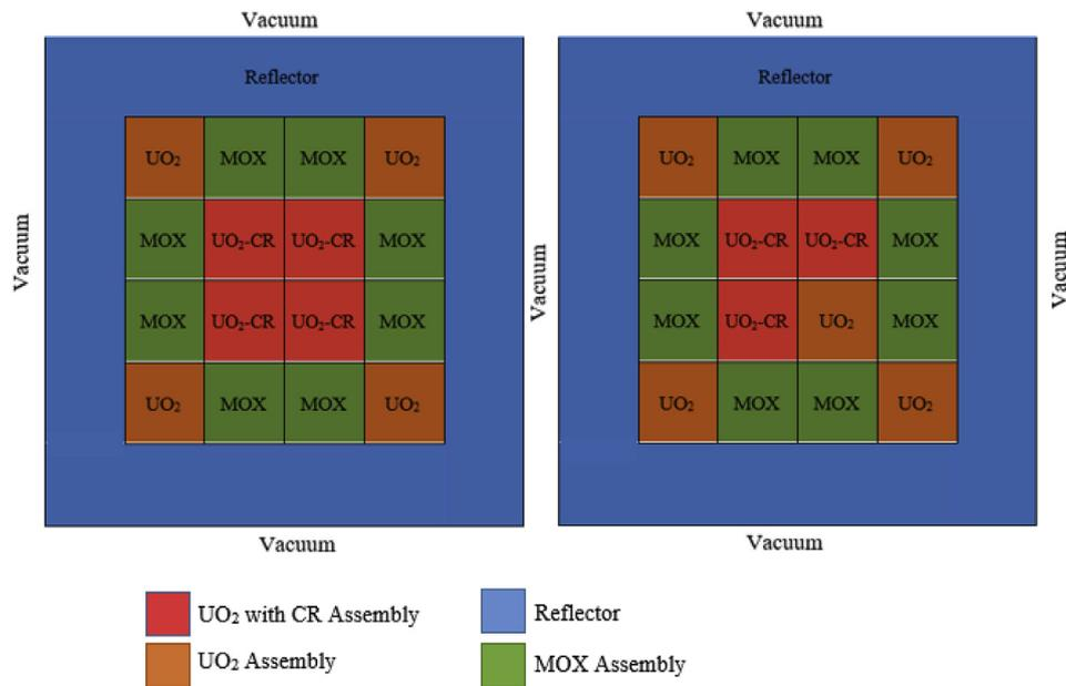
Fig. 13. Schematic of C5G7 core layout for the initial state (left) and final state (right).
