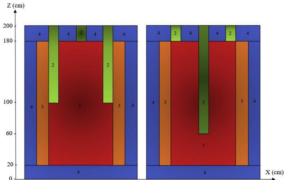
Fig. 11. Schematic of the LMW core layout for the initial state (left) and final state (right) on the X-Z page.
