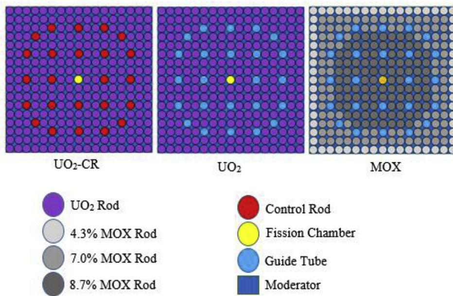
Fig. 14. Schematic of C5G7 fuel assembly layout.
