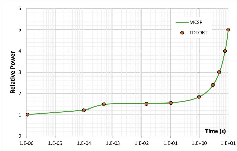
Fig. 4. Relative power vs. time for benchmark problem 16-A1.
