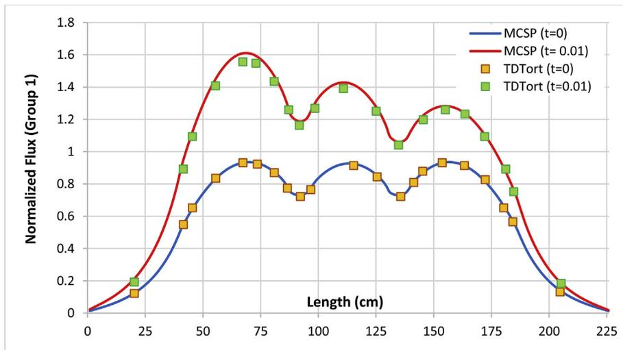
Fig. 5. Normalized flux vs. radial position for problem 16-A1 (group 1).
